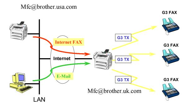
From the illustration above we can send an e-mail from any user connected to the LAN across the Internet which is then relayed to upto 48 different G3 fax machines. In order to stop unauthorised relaying of messages the Internet fax machine that is to relay the information needs to be configured to trust domains that it will allow access to the Relay feature.
